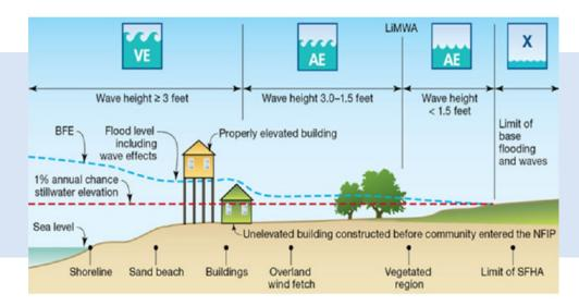
In the illustration, the dashed red line represents a 1% inundation level and the dashed blue line is the base flood elevation (BFE). These can be referenced to grade elevation. Zone definitions are provided at the top of the figure (VE, AE, LIMWA, and X).
